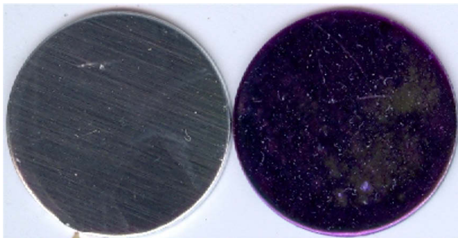
Figure 5. Unmodified, plasma-treated and plasma-treated and subsequently PAA-coated and washed substrates that were subsequently exposed to o-toluidine.
